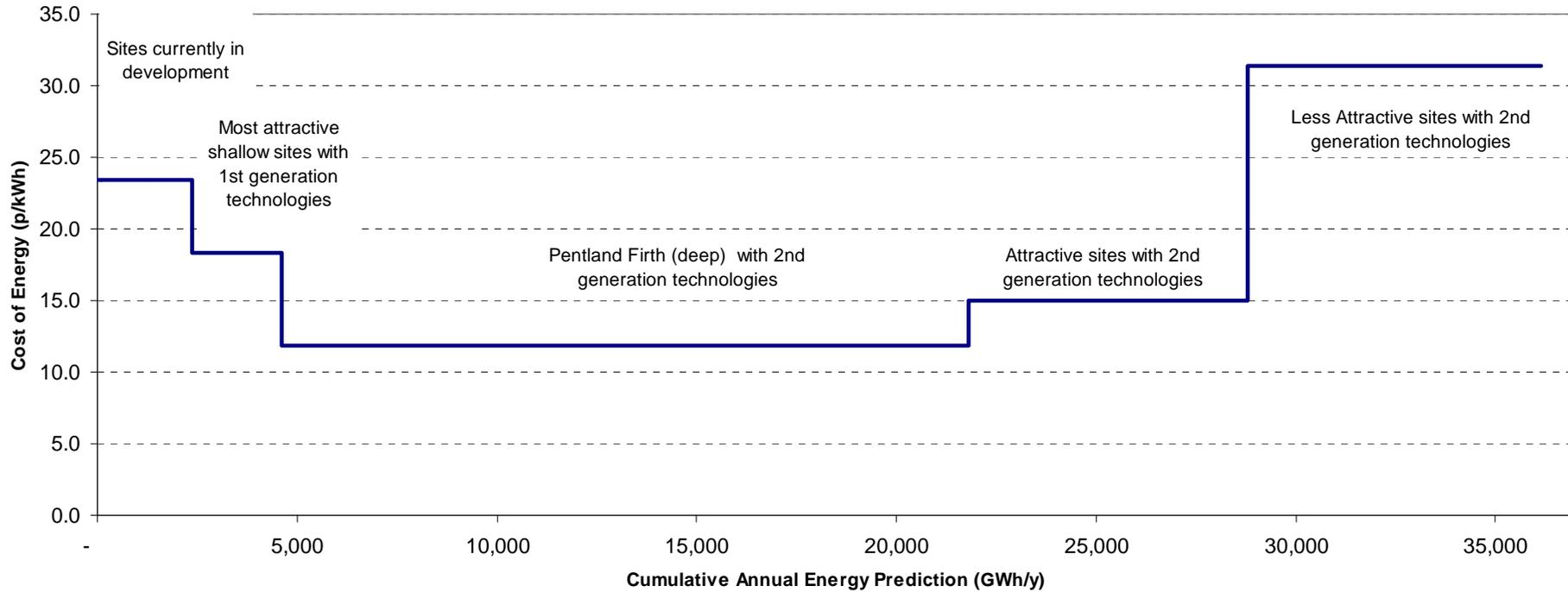
Figure 4-13 Black & Veatch 2011 model results: Cost-Resource curve with Pentland Firth optimised (P50 results only)
