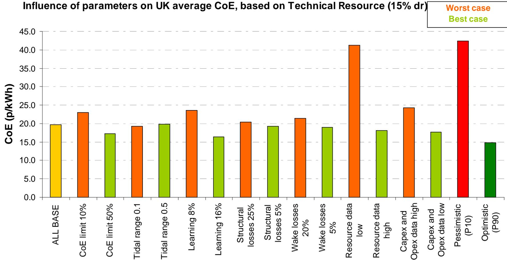
Figure 4-11 Sensitivity analysis on Cost of Energy
