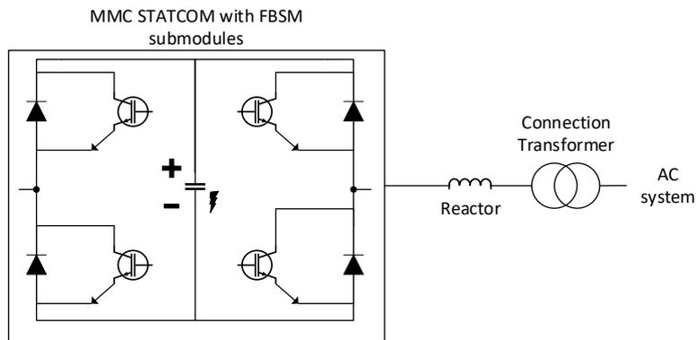
**Figure 2: Simplified schematic of a MMC submodule with embedded energy storage**
