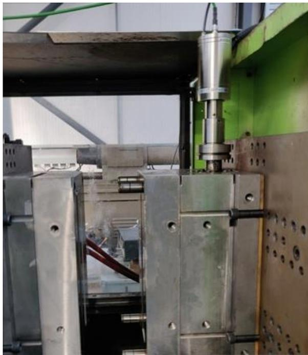
**Project description:** The project aims to demonstrate the three forms of Matrix Moulding Systems' Sonimelt technology, covering a wide range of applications in the injection moulding sector. The technology aims to decrease energy consumption through reduced melt and cooling electrical load, as well as reducing pressure requirements for the moulding of plastic parts on cold and hot runner systems.
